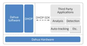
Dahua Open Platform (DHOP) is an open application platform that allows 3rd party applications to be downloaded and installed on Dahua Network Cameras.
